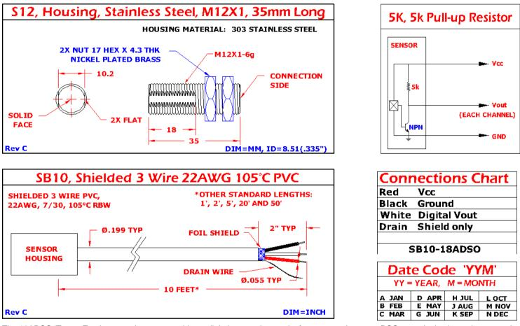
The 18ADSO 'Target Tracker speed sensor provides a digital output that tracks ferrous metal targets. DSO type single channel sensors do not require orientation to the target and will detect standard ferrous gears from 0 - 32 pitch. These sensors are also ideal for the detection of gears with uneven tooth spacing, detecting holes in rotating discs, or the detection of other targets such as bolt heads, studs, or other ferrous features on rotating targets.
