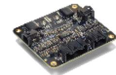
CMU 100819 *) isoSPI connector at side Balancing current 75mA (@4.2V)
