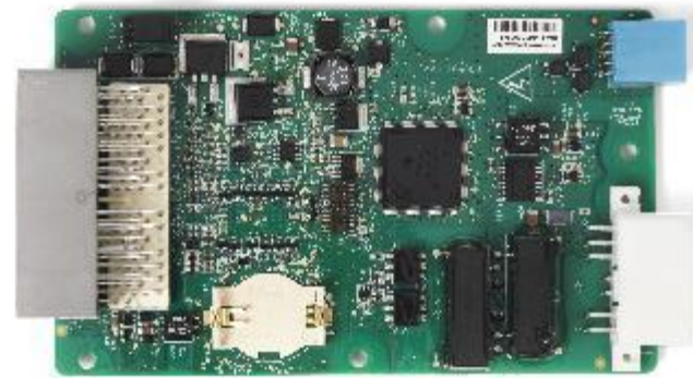
MCU – Master Control Unit
